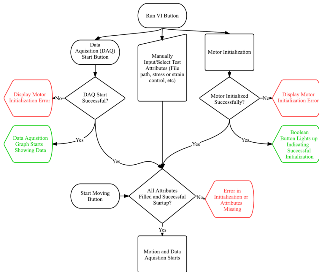
Figure 7. Logic state chart for initialization steps with indications where errors would occur and signal
