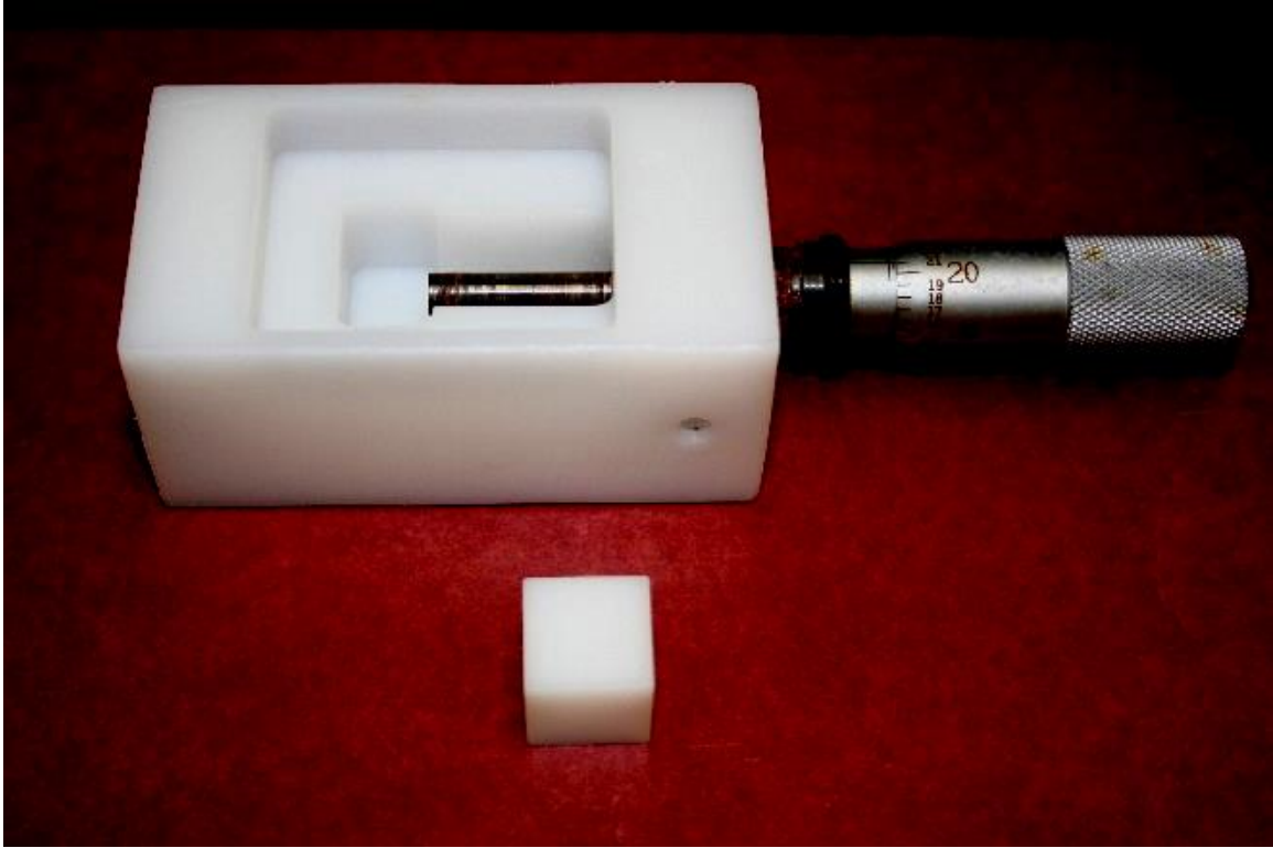
Figure 3. Initial strain application method involved manually spinning a micrometer to apply specific strains by compressing cartilage against a polyethylene block. The strain was held constant for one hour.
